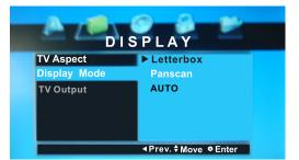
4.TV Output is used to switch TV system when you need . Here provide PAL, AUTO, and NTSC. When connect to TV set, choose TV system according to actual situation until get satisfied picture. In defect mode, choose NTSC.
